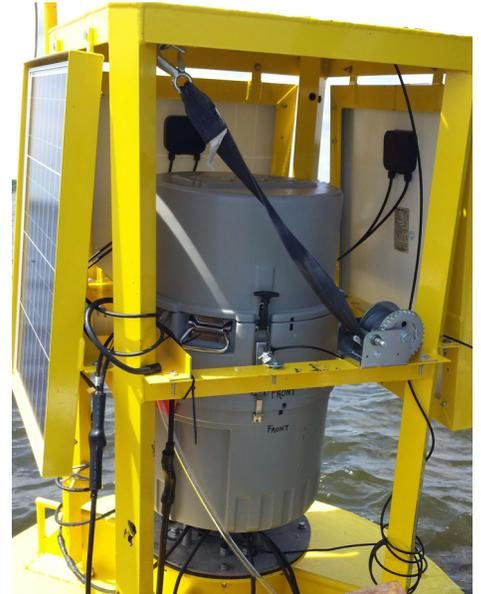
Sampler on buoy with solar panels
